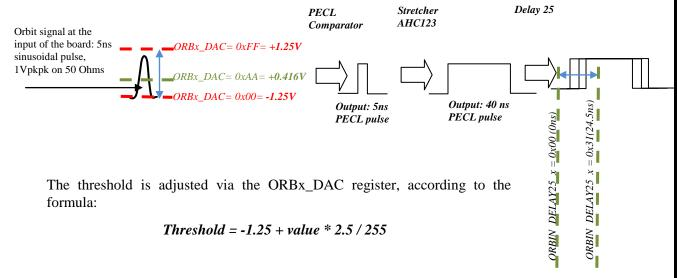
The ORBx\_DAC registers are set to 0xAA by default (which corresponds to 0.416V). This value should match perfectly with the level of the input signals. However, if you have any doubt or you want to adjust it better, we advise you to respect the following procedure. 'x' = '1' or '2'.
