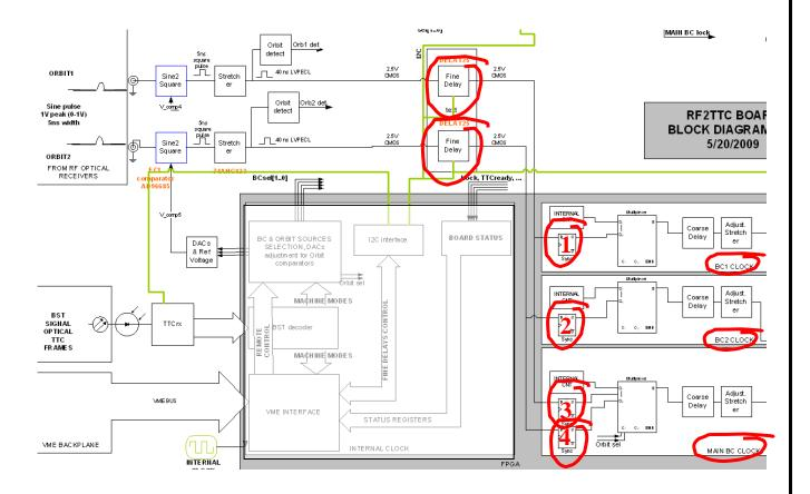
As the phase between the orbit and its relative BC is not known when it enters the latch in the FPGA, we may face a problem of metastability if the rising edge of the orbit pulse occurs close to the rising edge of the BC. This metastability window is in a range of [-setup time; +hold time] of internal FPGA flipflops, which should be of the order of max [-1ns;+1ns] (see graph below). Although very unlikely to happen, this situation <u>must</u> be avoided, and a calibration is recommended.
