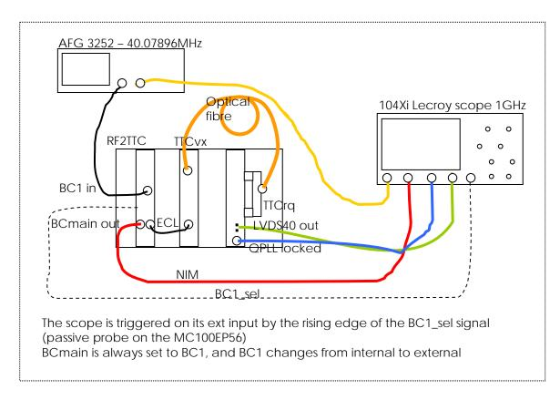
Differences with the setup1: although the source of the signal is connected to BC1, the QPLL of the RF2TTC involved in this test is the BCmain QPLL. The delays between the BC1 and its QPLL, and BC1 and BCmain QPLL are different. In this case, we can often see a loss of lock of the QPLL on the TTCrq (the TTCrq is the same for the 2 setups).
