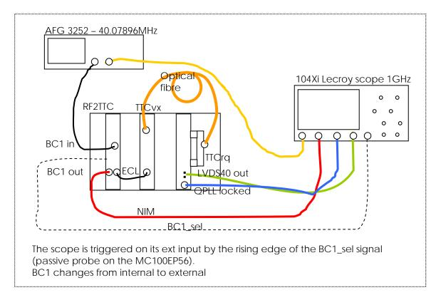
Signal analysis after a BC1 source change (internal=40.0784MHz, external=40.07897MHz). (BC1\_sel register value changes from 0 to 1)
