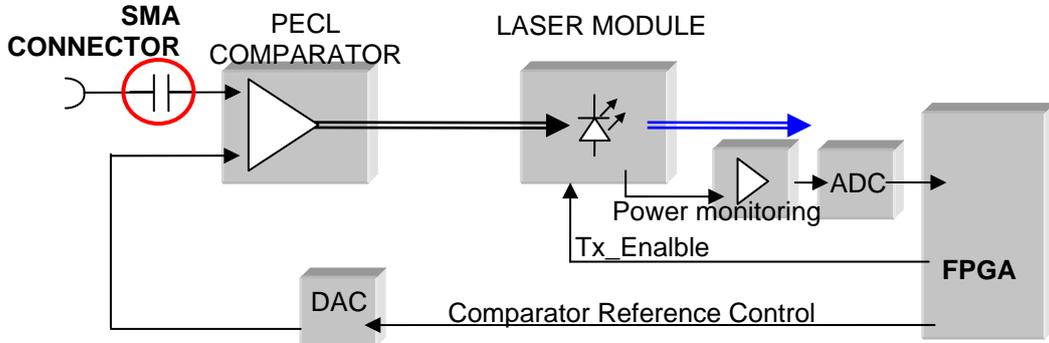
Picture 2.2.b: Optical Interface Diagram
