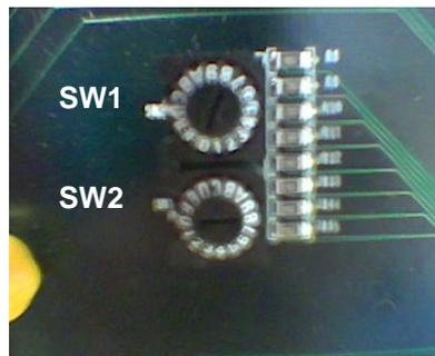
Picture 2.3: Module address selector
