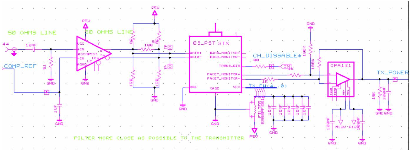
Picture 2.2.c: Optical Interface schematic
