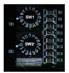
Picture 2.3: Module address selector
