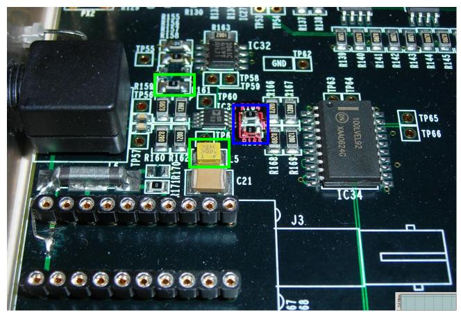
Picture 2.3.3.3e: Truelight Selection – Vref controlled by FPGA/VME (0R0) + Inductance
