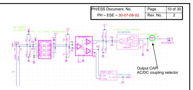
Picture 2.2.2: Photodiodes Post-Processing Logic
