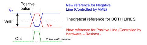
Picture 2.3.3.3c: Positive pulse in an Unbalanced Thevenin network
