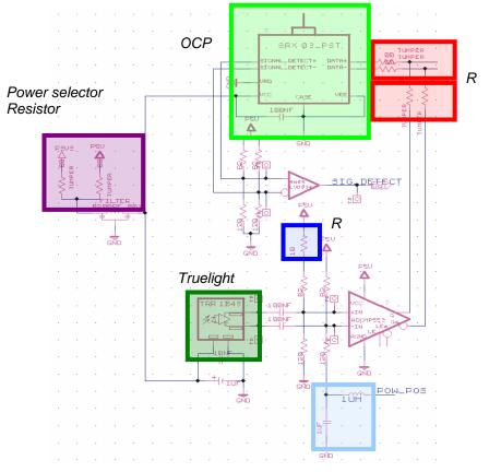
Picture 2.2.1.a: Photodiodes Module in EDA 1382
