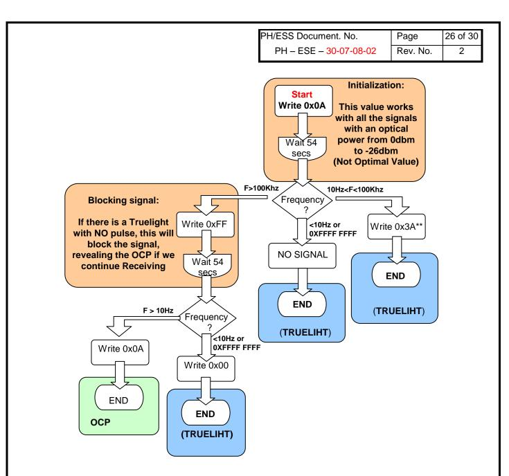
Picture 2.4.3: Remote Calibration Procedure
