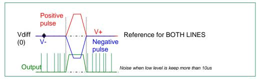
Picture 2.3.3.3b: Positive pulse in balanced Thevenin network
