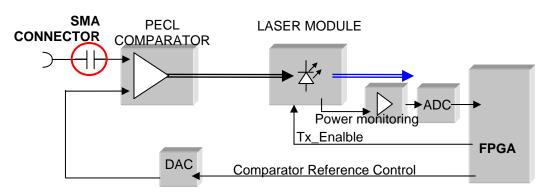
Picture 2.2.b: Optical Interface Diagram
