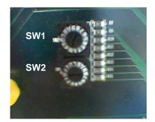
Picture 2.3: Module address selector
