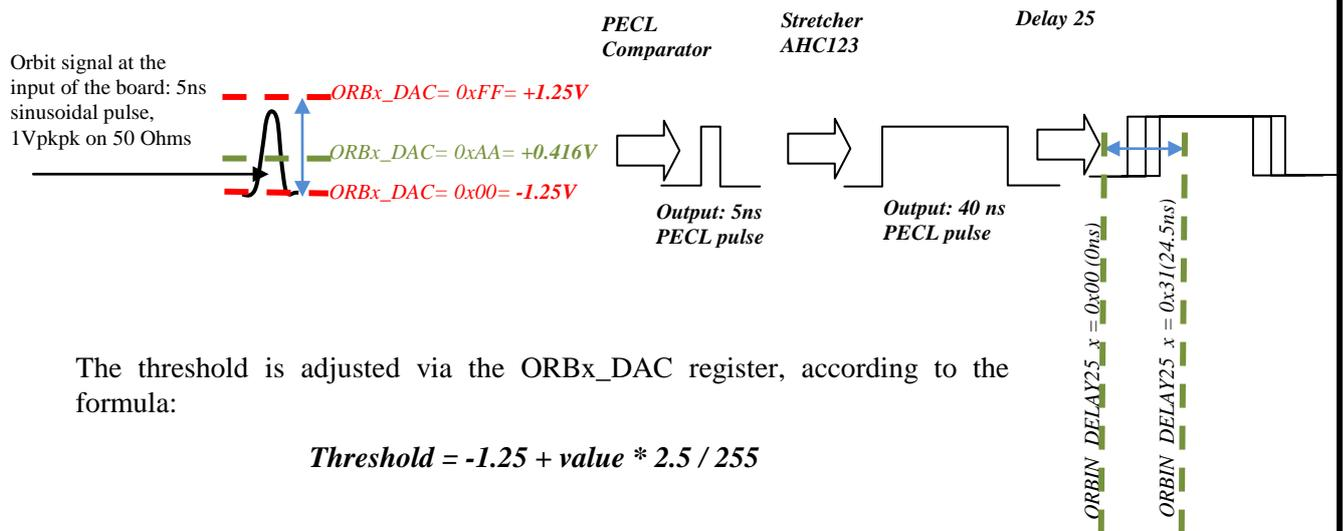
The threshold is adjusted via the ORBx\_DAC register, according to the formula:
