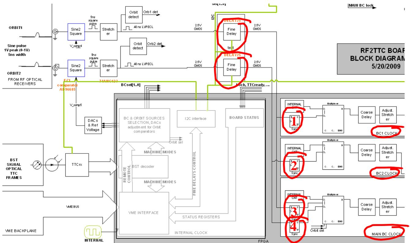
As the phase between the remote orbit and its relative BC is not known when it enters the latch in the FPGA, we may face a problem of metastability if the rising edge of the orbit pulse occurs close to the rising edge of the BC. This metastability window is in a range of [-setup time; +hold time] of internal FPGA flipflops, which should be of the order of max [-1ns;+1ns] (see graph below). Although very unlikely to happen, this situation must be avoided, and a calibration is recommended.
