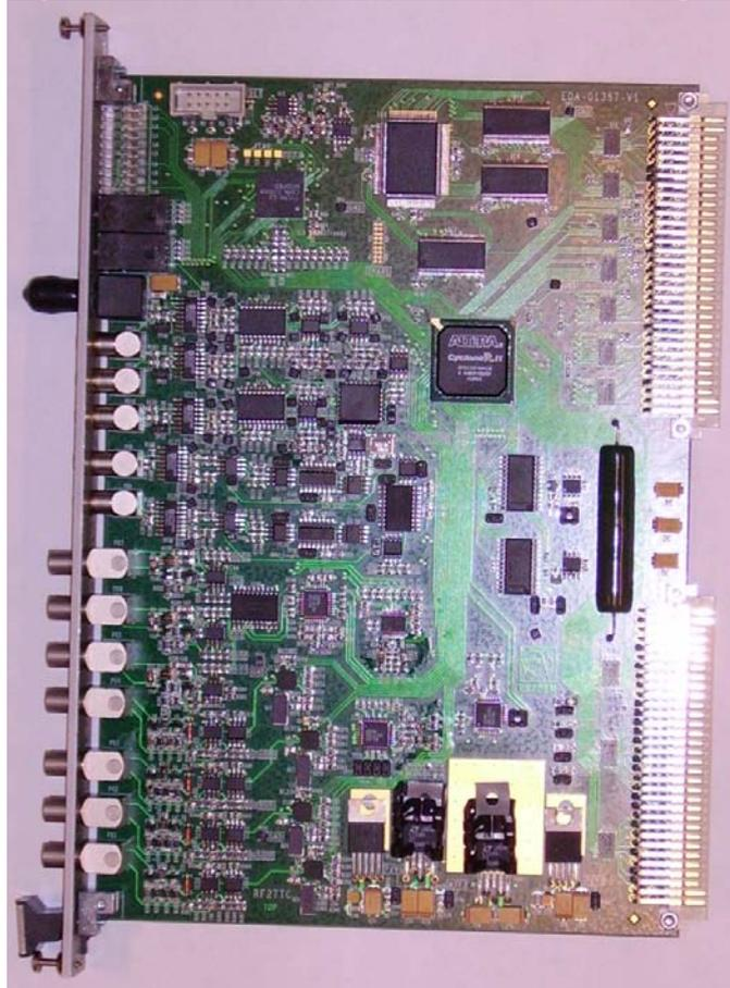
The timing signals treated by the RF2TTC are the three 40.078MHz Bunch Clocks (BC1, BC2 and BCref) and the two orbit signals (Orb1 and Orb2) necessary to drive the 2 beam lines of the LHC. The RF2TTC module converts them into ECL signals, and performs various adjustments on each signal before making them available for the in-detector TTC electronics.
